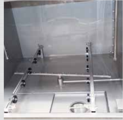
Rotating spray boom from above and rotating spraybar from below.
