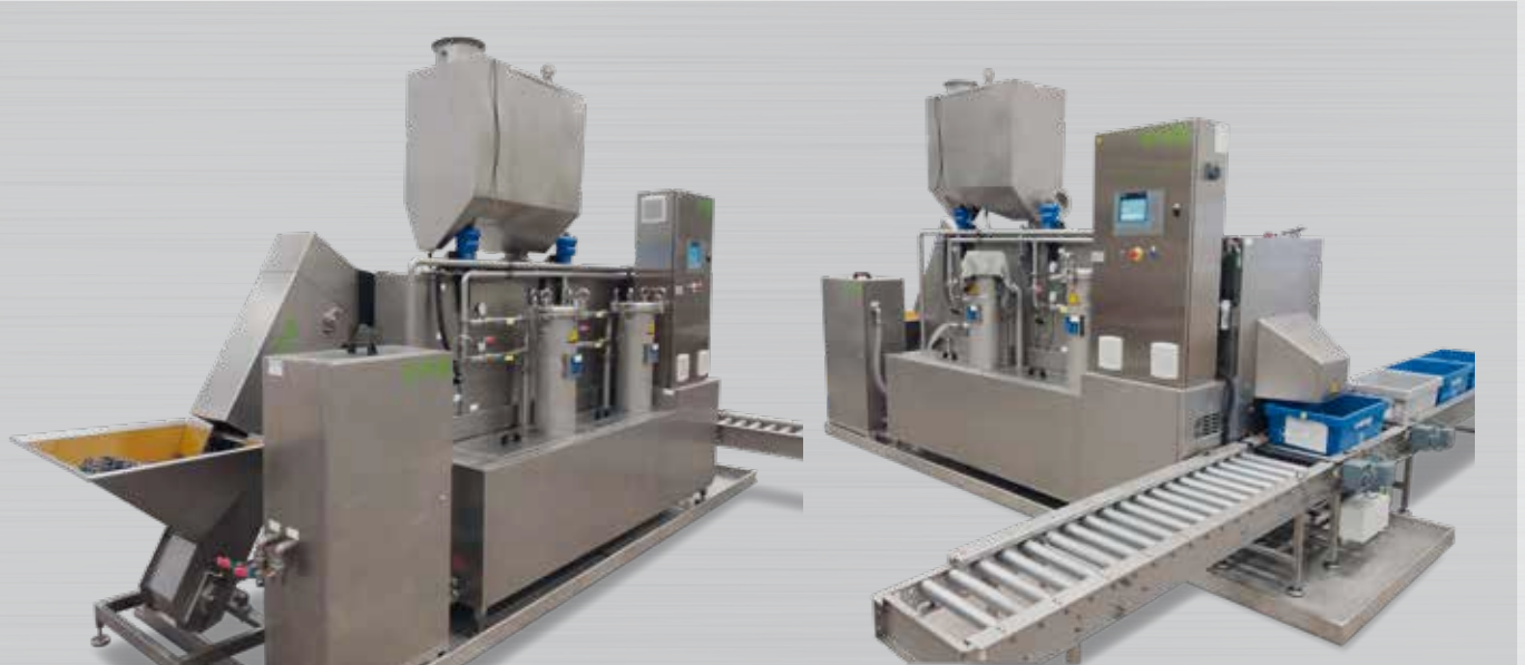
DC 1040 - wash/rinse/drying with feeder at inlet and conveyor belt with weight sensor at outlet.
